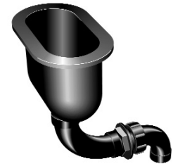
0476-BP Black Poly Molded of black polyolefin resins. Complete with 90° union elbow. Designed to be mounted in a vertical panel not over 1/4" thick. 6" x 3" inside dimension. 1 1/2" I.P.S. male straight thread outlet.
