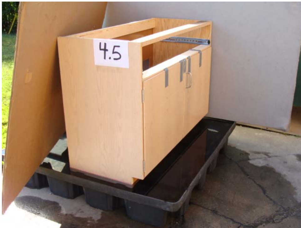
Photo 4: 4.5 Cabinet Submersion Test
