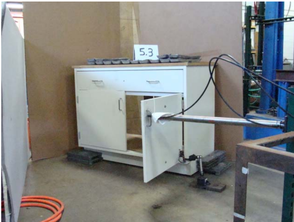
Photo 6: 5.3 Door Cycle Test
