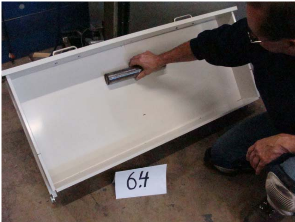
Photo 10: 6.4 Drawer Internal Impact Test
