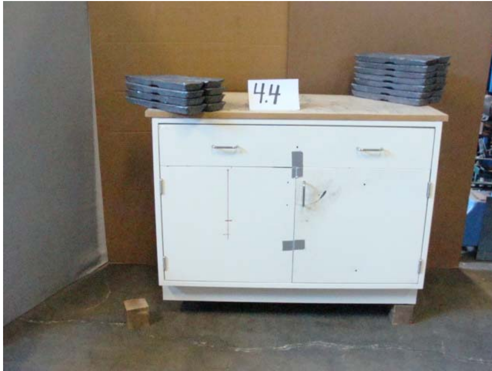
Photo 3: 4.4 Cabinet Torsion Test
